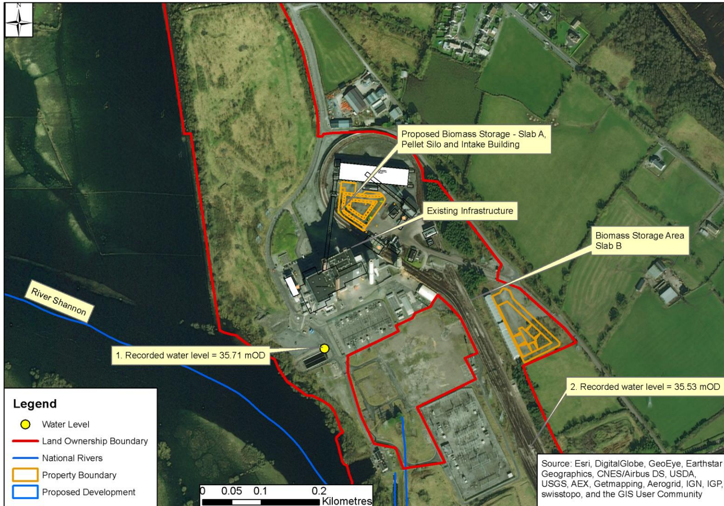
Figure 5-4 Recorded water levels during the November/ December 2009 flood event (levels provided by the OPW)
